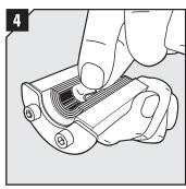
Adapt the seal to the cable/pipe by peeling layers from the halves until you reach the gap seen in pic.5.
