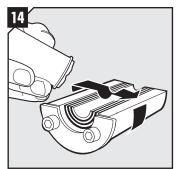
Lubricate thoroughly on the inside surfaces and sparsely on the outside of the seal with Roxtec Lubricant.
