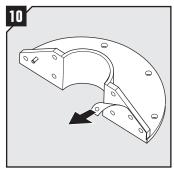
Remove the protecting tape of both sleeve halves.
