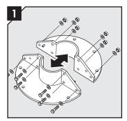
Clean the empty sleeve from dirt. Divide the sleeve by removing <u>all</u> bolts.
