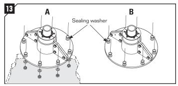
Fasten the sleeve to the floor by permanently fasten the rest of the bolts. Make sure the sealing washer on top side and gasket are in position. **B**: Washer and nut can be removed if the bolt holes are threaded. Thread hole: M10 23-75 and M12 100-644.
