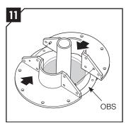
Assemble the sleeve around the cable/pipe. OBS: Gasket and sleeve joints shall not be at the same position.
