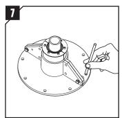
Use the sleeve as a template to mark out where to drill the bolt holes.
