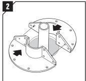
Assemble the sleeve around the cable/pipe. Let the guide pins located at the surface between the sleeve halves help you.
