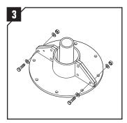
Preliminary fasten two of the bolts. One at each end of the sleeves flange. Do not tighten the bolts!
