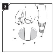
Remove the sleeve and the RS seal. Drill bolt holes. If you want, make threaded M10/M12 holes.
