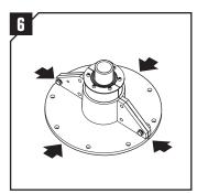
Center the sleeve to the cable/ pipe by partly inserting the RS seal into the sleeve.
