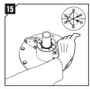
Insert the halves into the sleeve. Tighten the screws crosswise. The seal will compress and seal the transit. Please see table for recommended max torque.
