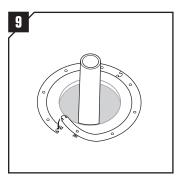
Assemble the gasket centered over the bolt holes. Fit the gasket parts into each other.
